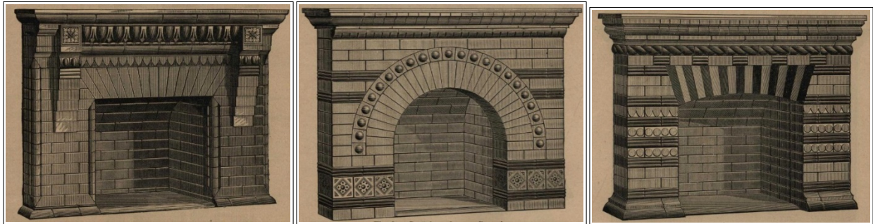
Figures 77, 78, 79: Example fireplaces from the 1890 Peerless Catalog , “ Isometrical Diagrams of Plain and Ornamental Bricks. ”
