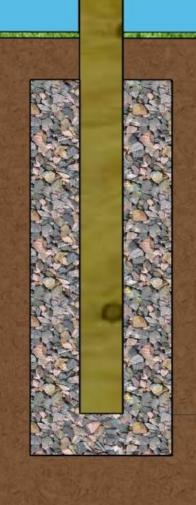
Each post is dug 3' into the ground with compacted gravel
