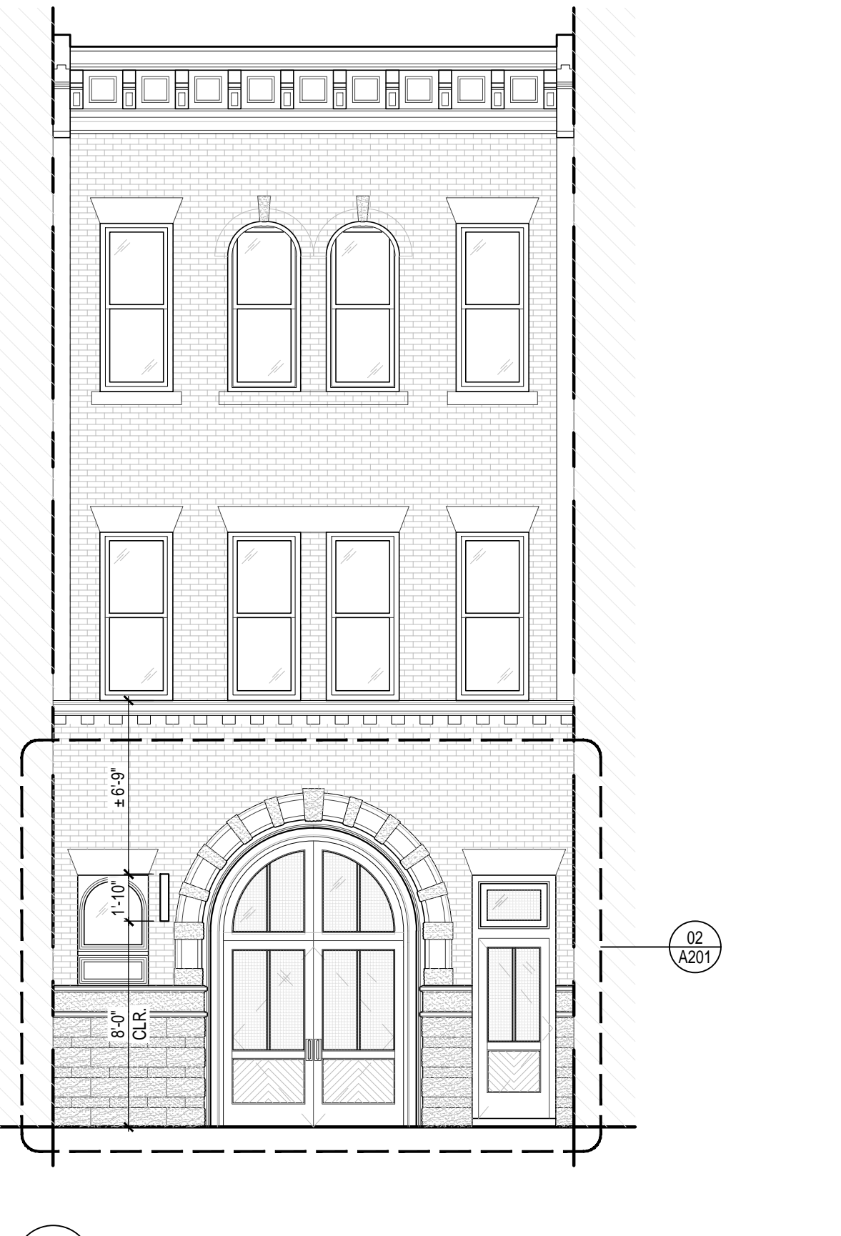
01 BUILDING ELEVATION KEY - SANSOM STREET FACADE 3/16" = 1'-0"
