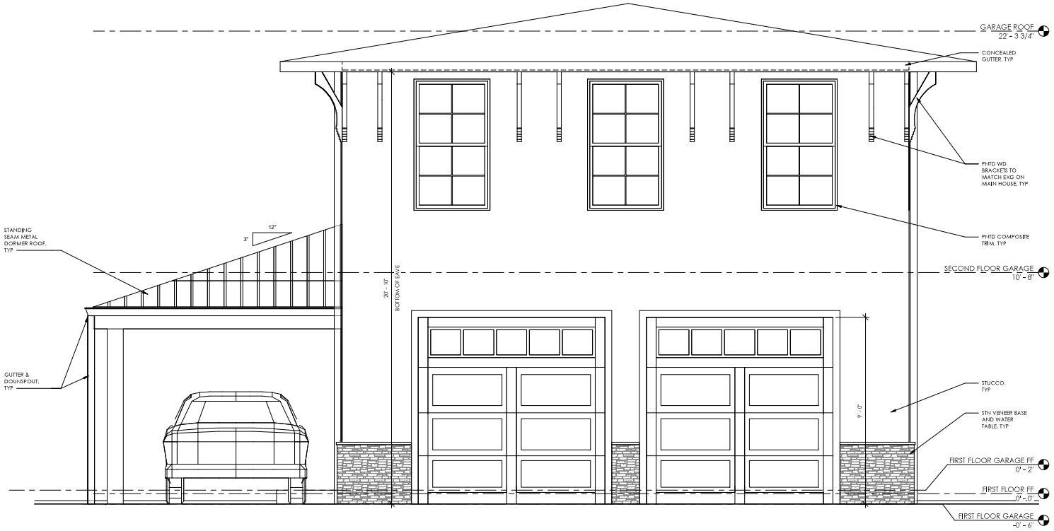
1 GARAGE ELEVATION SOUTH - B A3.8 1/2" = 1'-0"
