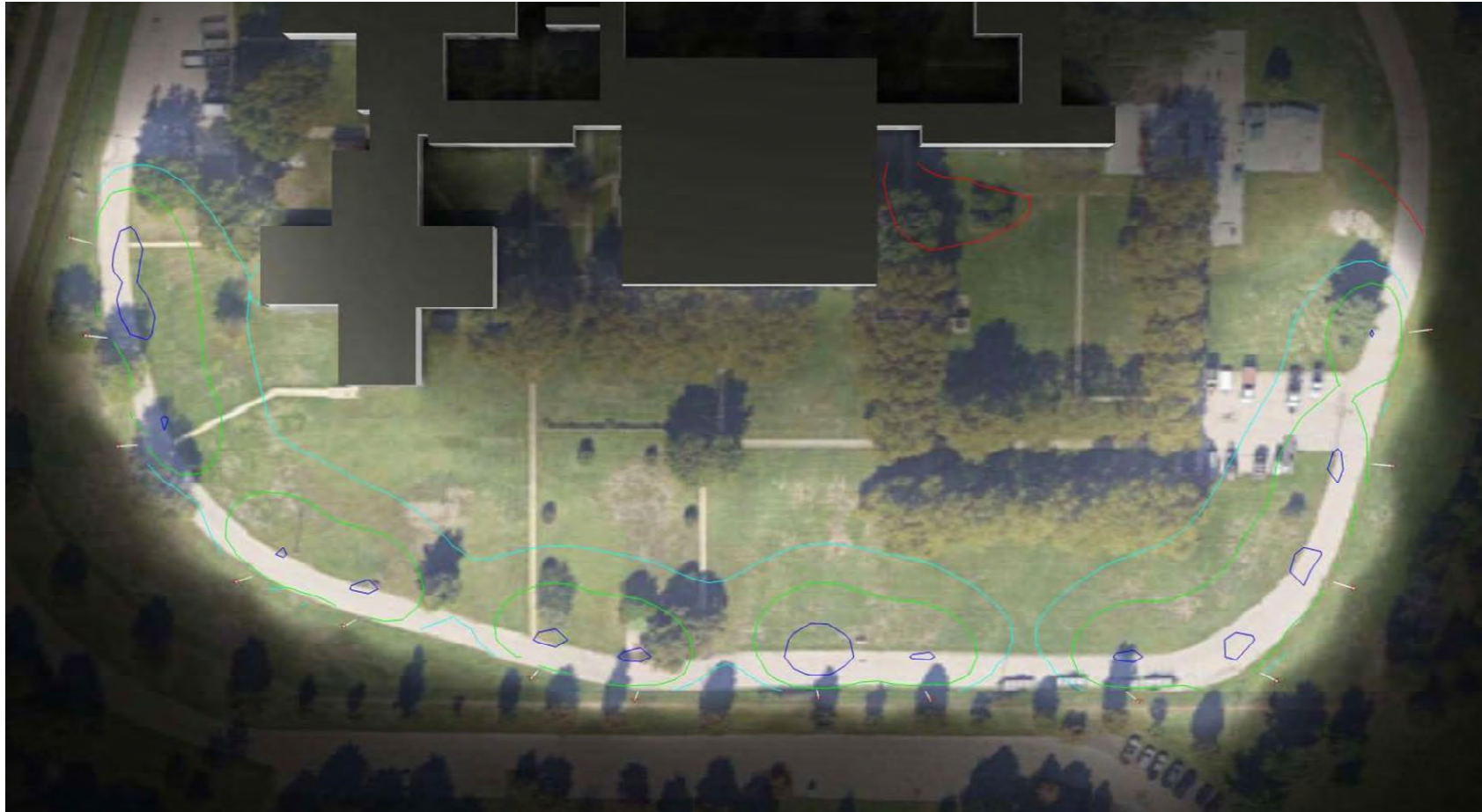
Perimeter Lighting Simulation
