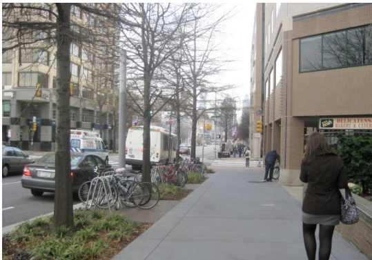
The furnishing zone provides a buffer from traffic and can accommodate bike parking, planters, and other amenities.
