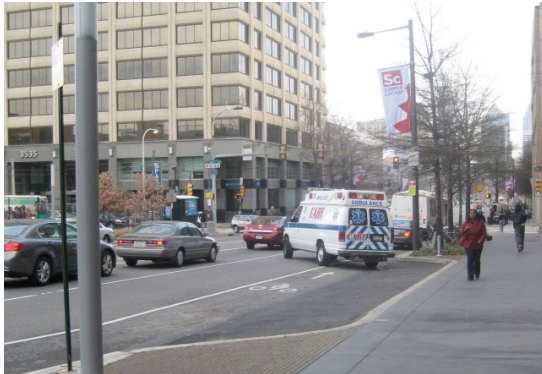
Lay-by lanes are generally discouraged because they allow vehicles to encroach into the sidewalk area and decrease comfort and safety for pedestrians (KAI).
