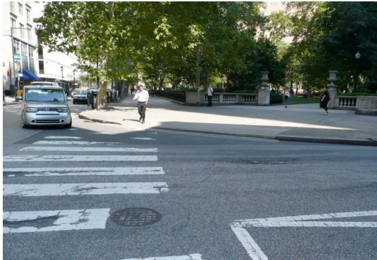
Large curb radii lengthen pedestrian crossing distances and allow vehicles to make turns at high speeds (KAI – Walnut St and Rittenhouse Square).
