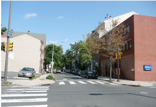
Continental crosswalks provide a high-visibility crossing treatment. (KAI – Signalized intersection S. Philadelphia)
