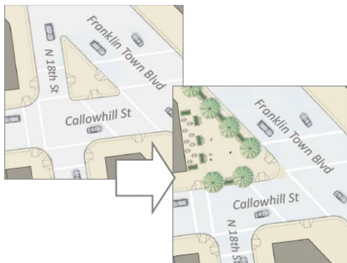
Complex intersections can be redesigned to eliminate conflict points and create an opportunity for public space and green infrastructure. (Adapted from San Francisco Better Streets Guide)
