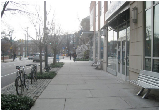
Minimum sidewalk width is 12' on most street types, including Walkable Commercial Corridors.
