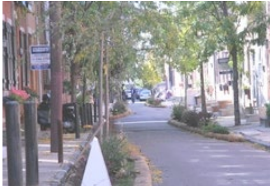
The Better Blocks Philadelphia project created temporary chicanes and other traffic calming features on Webster Street.
