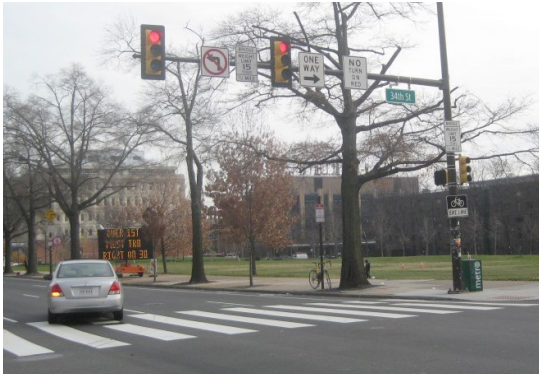
Posted (MUTCD R10-11) "No Turn on Red" signs are used to reduce conflicts between turning vehicles, pedestrians, and cyclists (KAI – 34th and Walnut)
