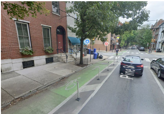
Green colored pavement in Pine Street bicycle lane.
