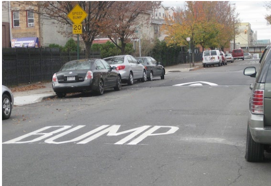
Signs and pavement markings should be used to warn approaching vehicles of raised speed reducers. (streetsblog)
