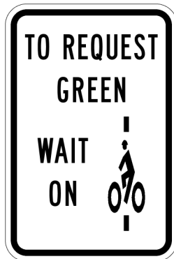
Bicycle detection should be provided at signalized intersections if the phase(s) serving bicycle movements is not set to recall each cycle. The “Bicycle Detector” pavement marking and sign (MUTCD 9C-7 and R10-22) should be used at intersections with in-pavement detectors.
