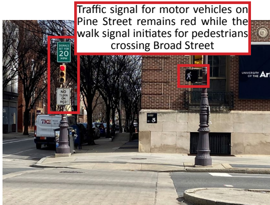
LPI at the intersection of Broad Street and Pine Street in Philadelphia (Source: KAI)
