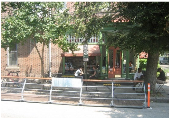
Railings, curbs, or delineator posts should be used to protect flexible parking lane uses from errant vehicles.
