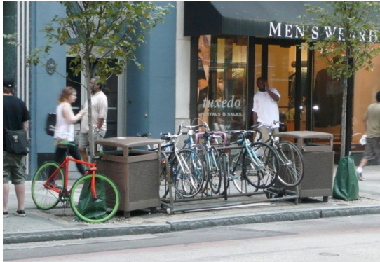
Unlike “inverted U” or “staple” racks, many older bike rack styles do not allow both the frame and wheel of a bicycle to be easily locked to the rack.
