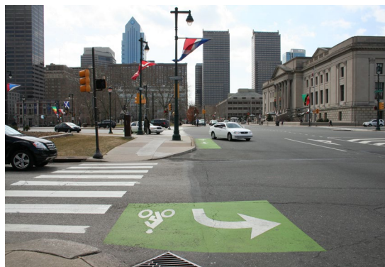
Two-stage left turn boxes provide a waiting area for cyclists at intersections where it is difficult to cross multiple lanes of traffic to make a left turn.
