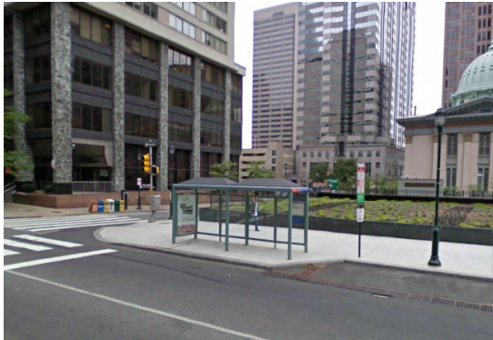
Curb extensions can be used to separate transit stops from the sidewalk clear zone. (18th and JFK)
