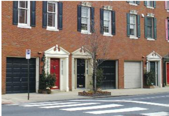
Many streets and homes in Philadelphia were not designed to accommodate driveways. Curb cuts can actually reduce overall parking capacity by eliminating on-street parking spaces. (PPC Rowhouse Manual).
