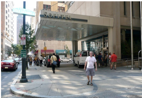
Driveways onto major streets should be limited, particularly in high pedestrian traffic areas, due to conflicts created with pedestrians and vehicles.
