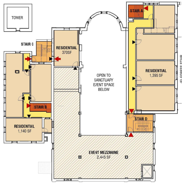
02 SECOND FLOOR PLAN 17'-0" x 10'-0" 2.22.2023 (R) BY: TOWER NOT INCLUDED
