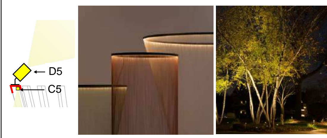
6 TYPE C5 & D5 C5 LINEAR ACCENT AND D5 TREE UPLIGHT INTEGRATED INTO TREE CAGE STRUCTURE
