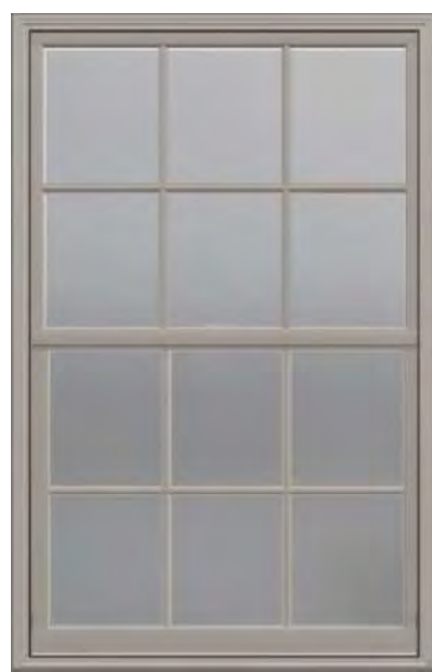
PROPOSED NEW DOUBLE-HUNG EQUAL SASH, SANDTONE EXTERIOR FULL-DIVIDED-LIGHT GRILLES 3x2 PER SASH SIZE: 32 5/8 "x51 1/4 " (SAME AS EXISTING) 3 UNITS WITH THIS SIZE/AESTHETIC
