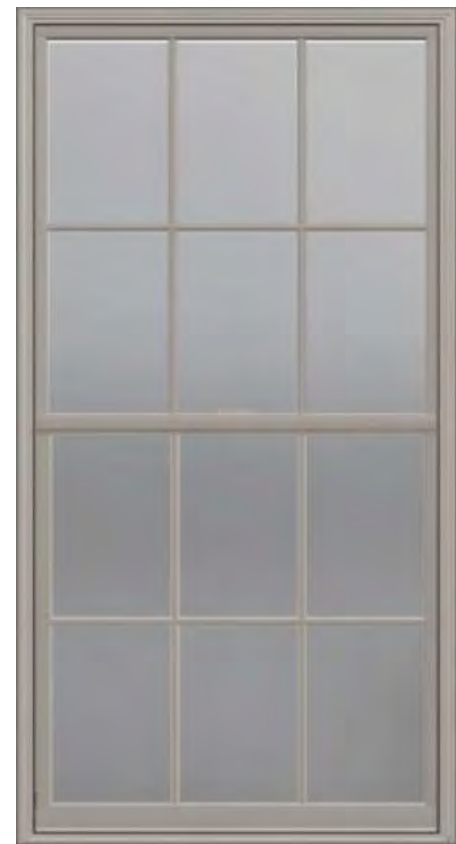
PROPOSED NEW DOUBLE-HUNG EQUAL SASH, SANDTONE EXTERIOR FULL-DIVIDED-LIGHT GRILLES 3x2 PER SASH SIZE: 35 5/8 "x68 7/8 " (SAME AS EXISTING) 2 UNITS WITH THIS SIZE/AESTHETIC
