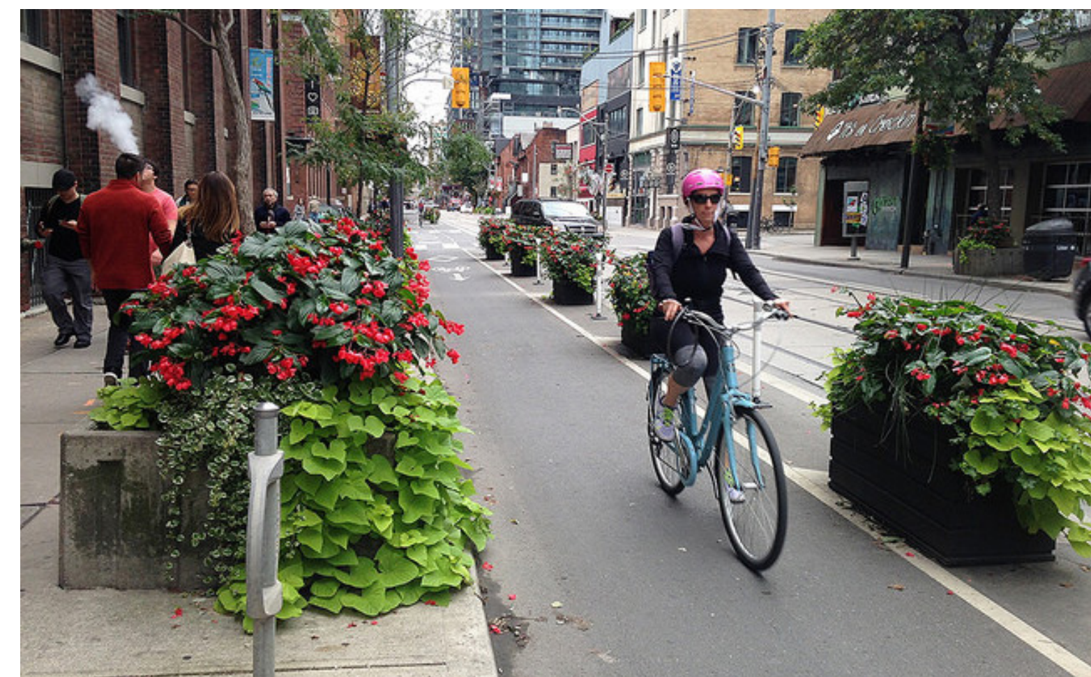
Example of a bike lane separated with planters in Toronto. The City is working out planter maintenance details with partners.
