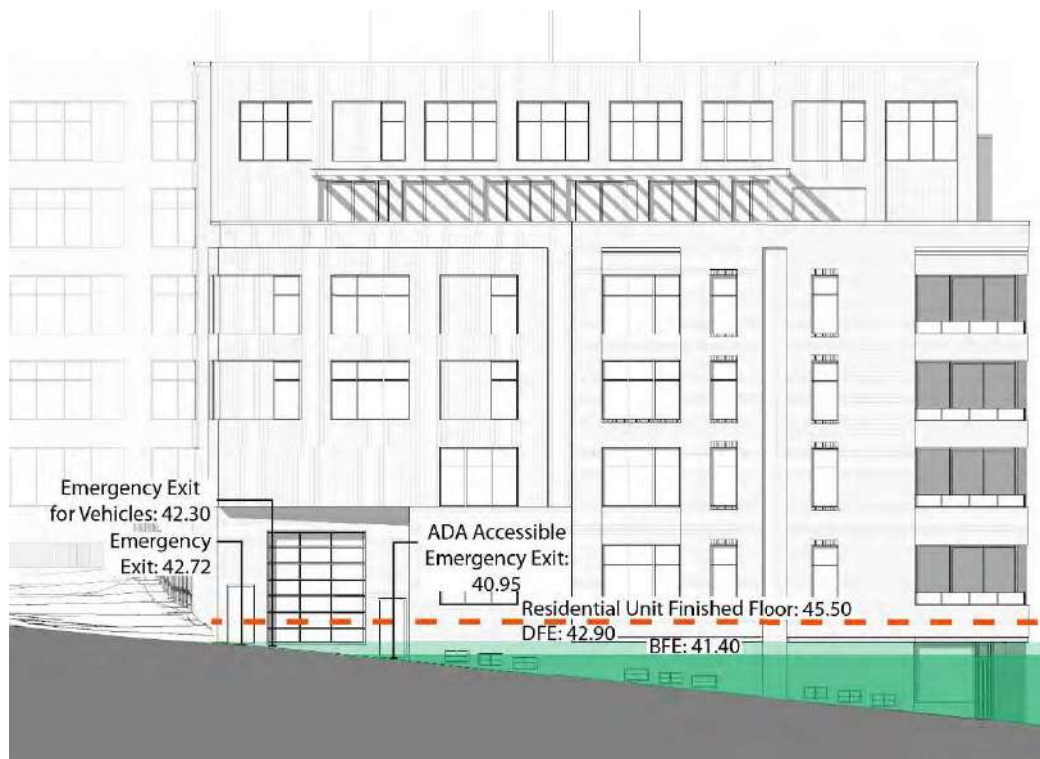
Figure 2: Elevation view of west building (per CBP Architects 6/06/24 plans) with key flood and building elevations
