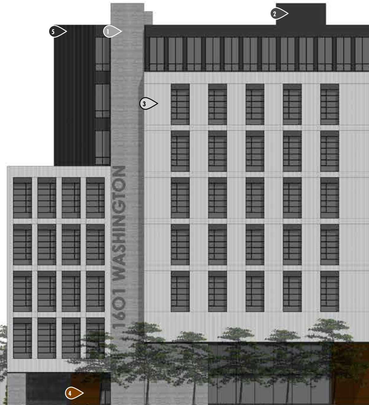
3 LIGHT CORRUGATED METAL PANEL LIGHT GRAY ALUMINUM COMPOSITE PANEL WITH CORRUGATED FINISH, VERTICAL APPLICATION
