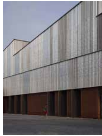
3 LIGHT CORRUGATED METAL PANEL LIGHT GRAY ALUMINUM COMPOSITE PANEL WITH CORRUGATED FINISH, VERTICAL APPLICATION
