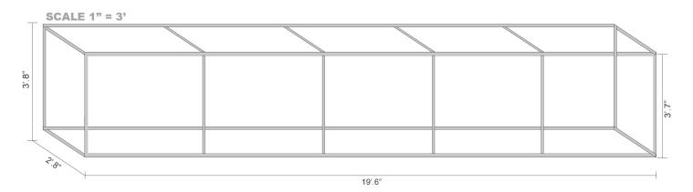
SIGN BOX STRUCTURAL FRAME SYSTEM: 1"X 1"X3/16" Galvanized Steel Tubing W/ Welded Connections.
