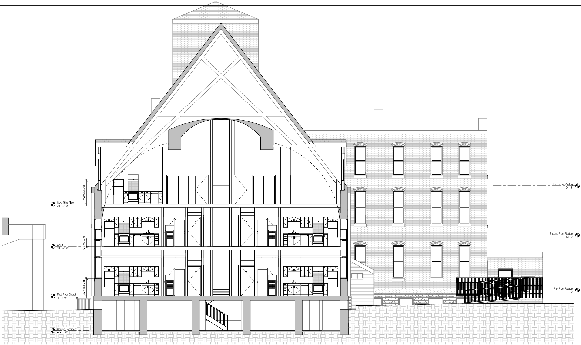
1 Transverse Building Section Through Church 1/4" = 1'-0"
