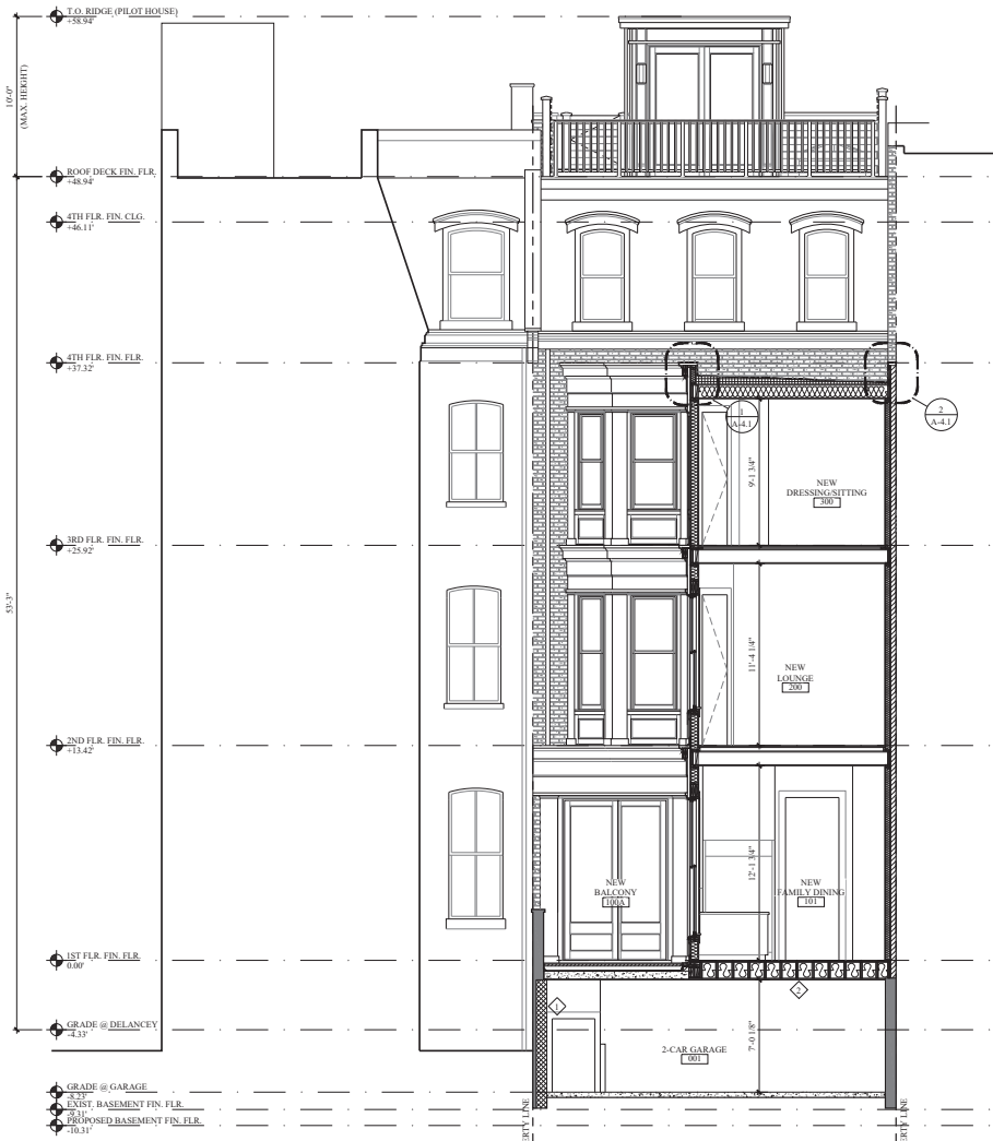
2 A-3.0 PROPOSED BLDG. SECTION @ ADDITION SCALE: 1/4"=1'-0"
